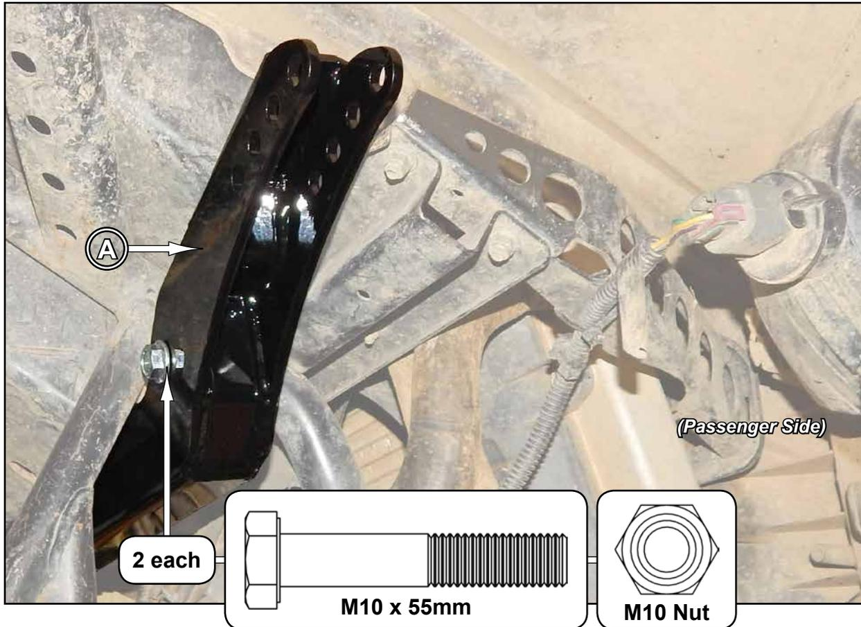
Use above hardware or stock hardware when installing Shocks.
