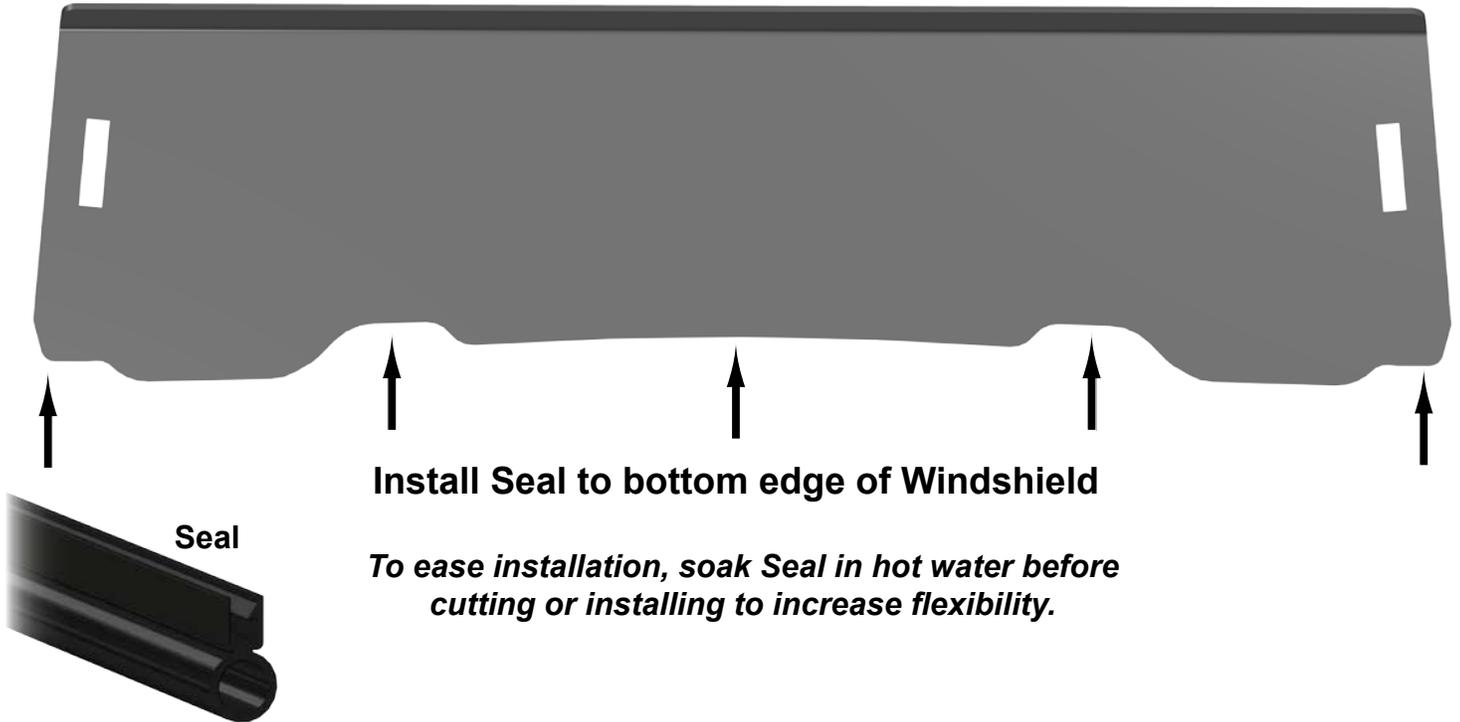
**Install Seal to bottom edge of Windshield**
