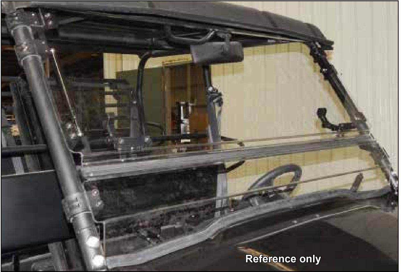
**Install Seal along bottom edge of Lower Windshield (B)**
