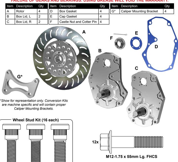
Installer must reference machine specific Portal Gear Hub installation instructions at Superatv.com.
