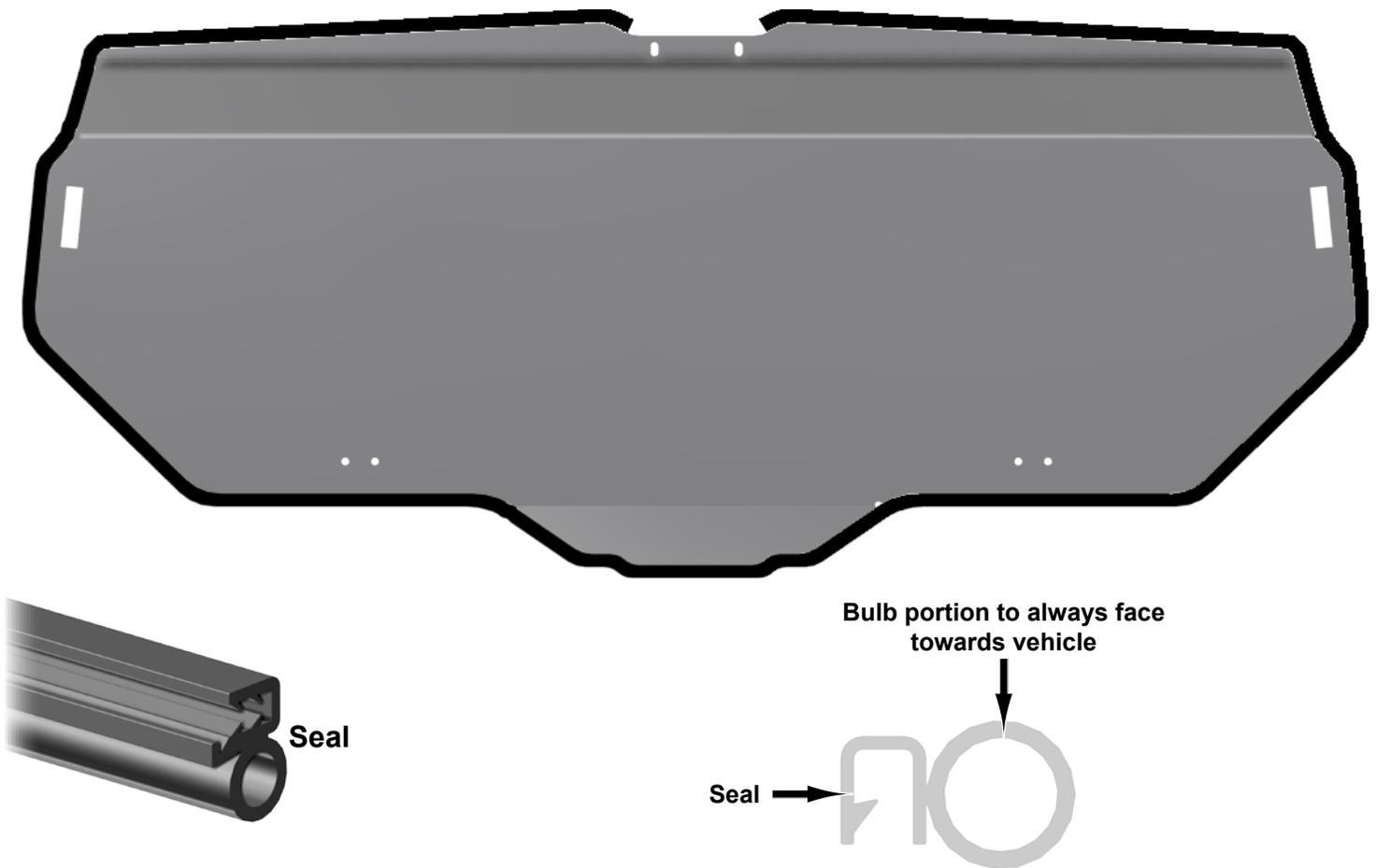
***To ease installation, soak Seal in hot water before cutting or installing to increase flexibility.***
