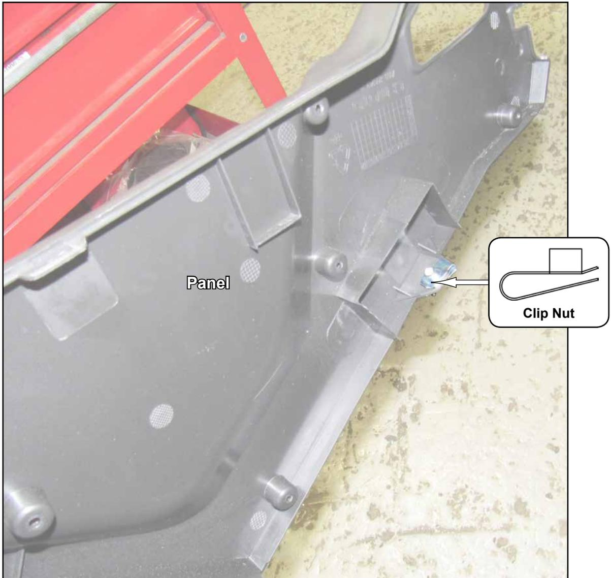
**do not tighten hardware completely**
