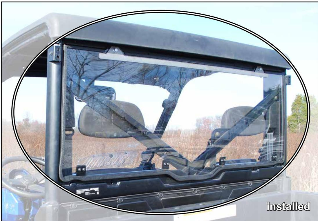
**Install Seal to Windshield (A) as shown:**
