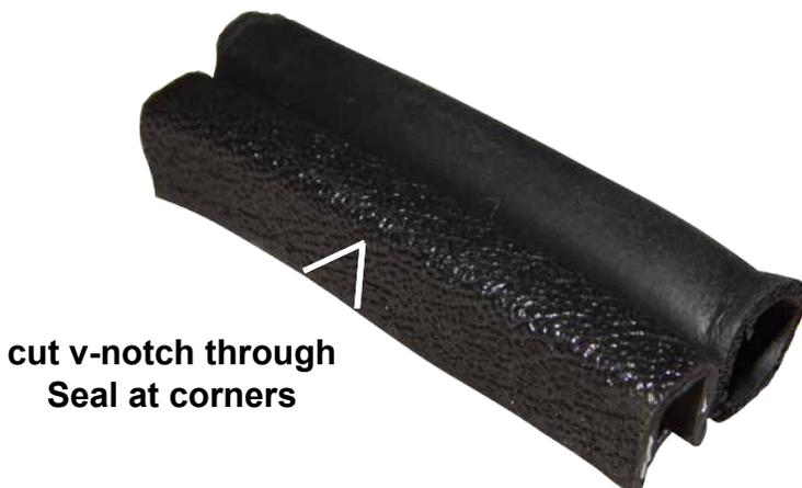
**Cut only to inside of channel when cutting v-notch**
