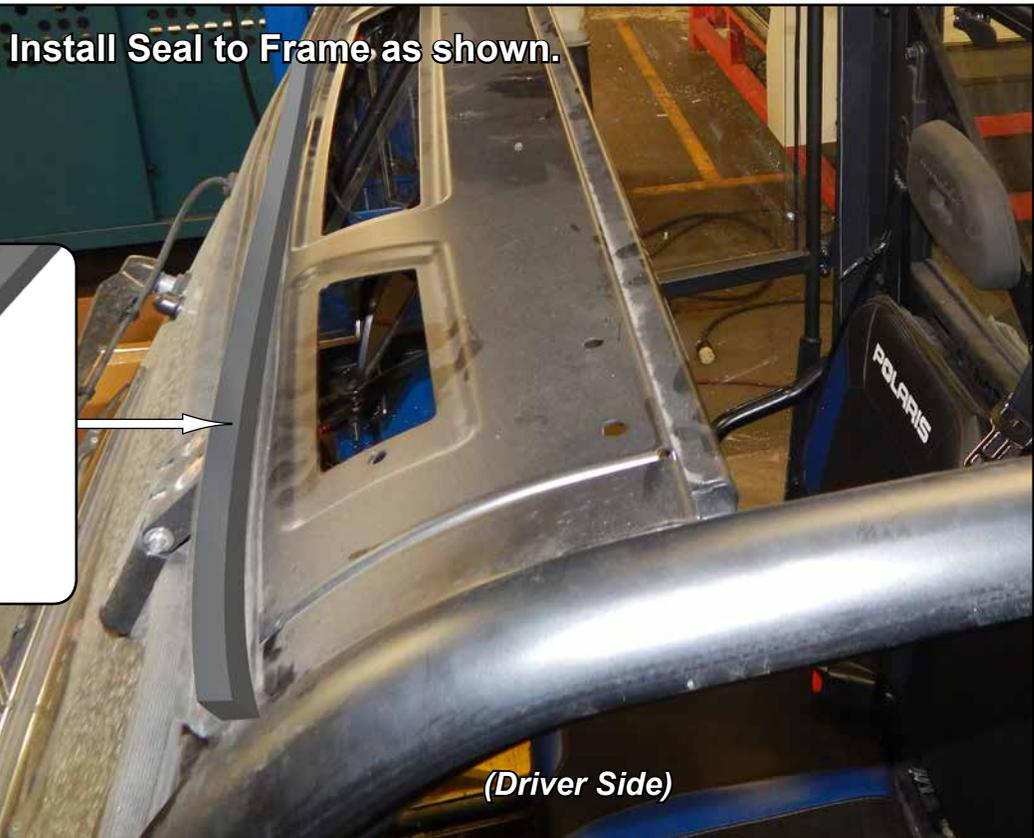
When installing, do not tighten any hardware completely unless noted.
