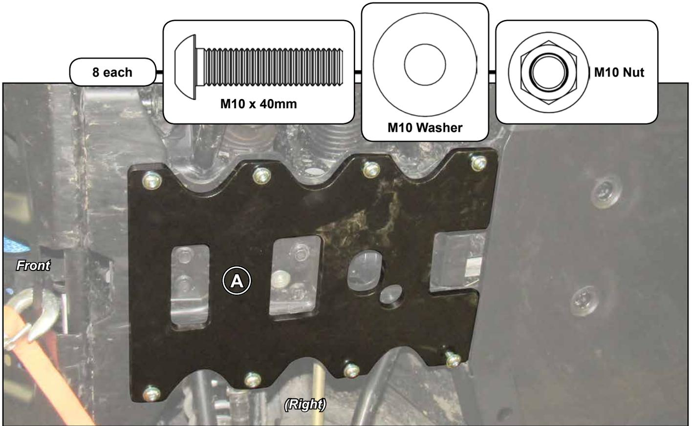
tighten hardware completely
