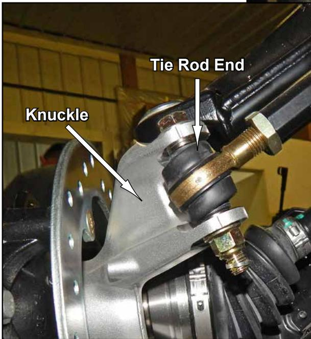
Tip: rotate Knuckle and use setup shown when removing/installing from Upper Arm.
