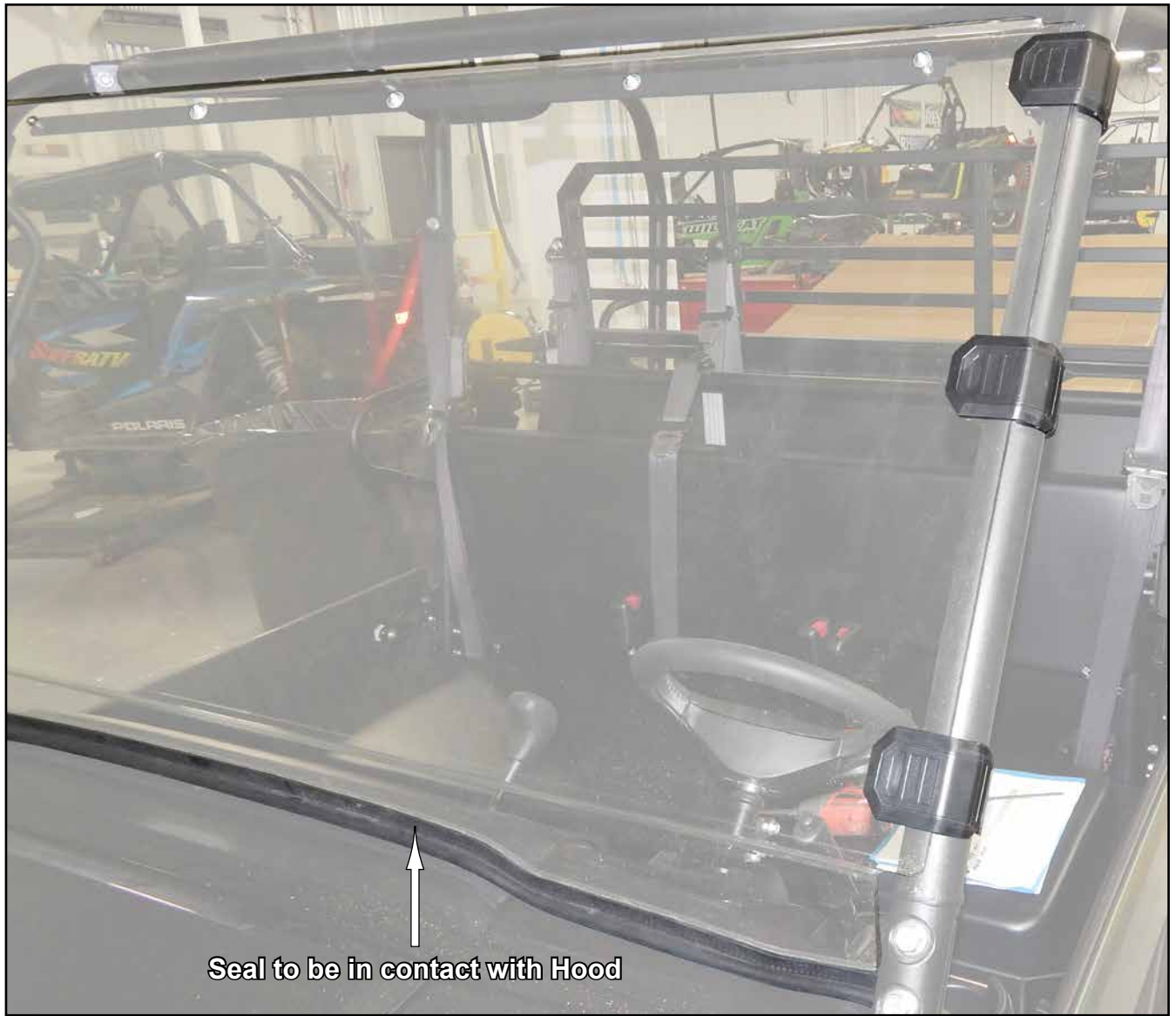
Insert Clamps into slots in Windshield...
