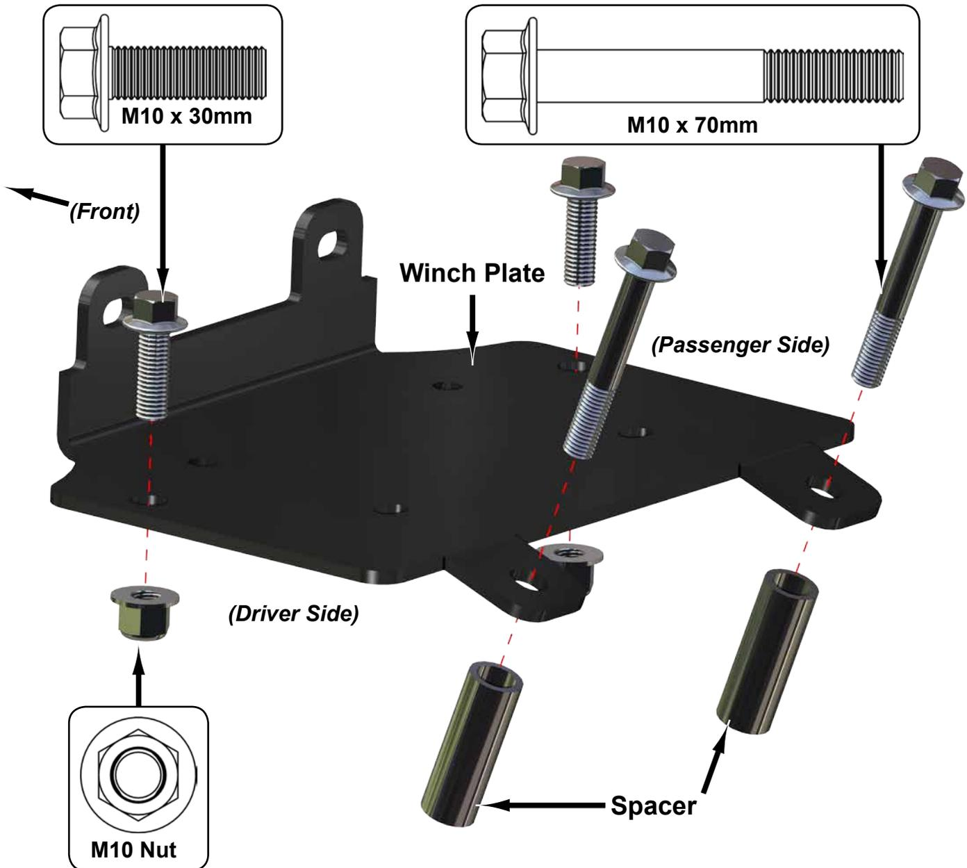
**Remove Skid Plate hardware shown before installing Winch Mount.
