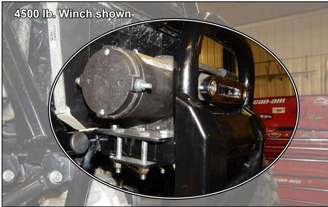
**! Install 3500 Fairlead Adapter (B) if using a 3500 lb. Winch**
