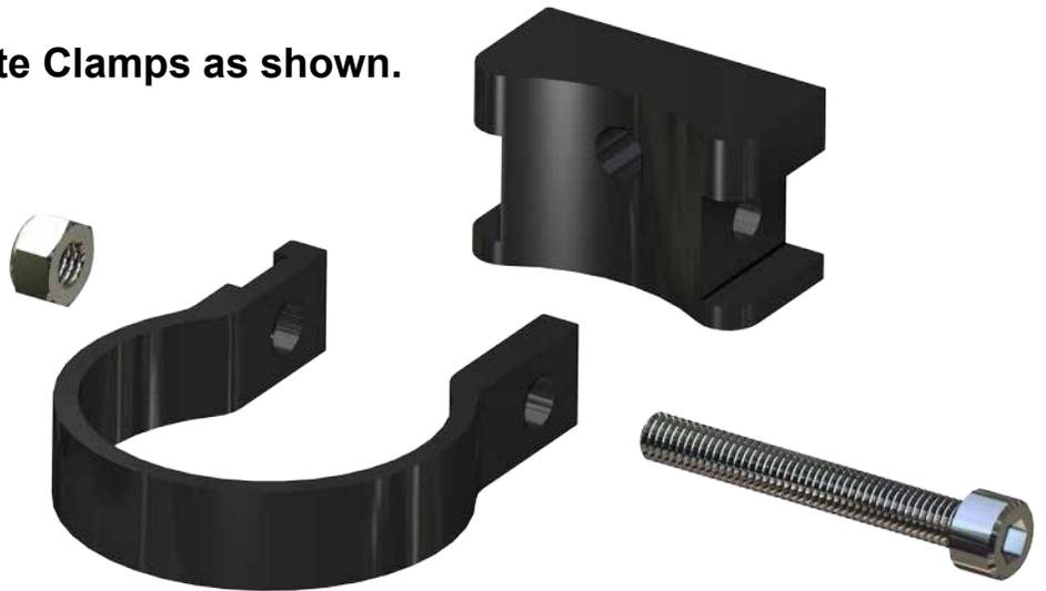
**Cut and install Foam to Clamps as shown.**
