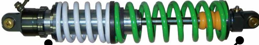
**Do not set Compression Adjustor to full clockwise position. Shock failure will occur.**
