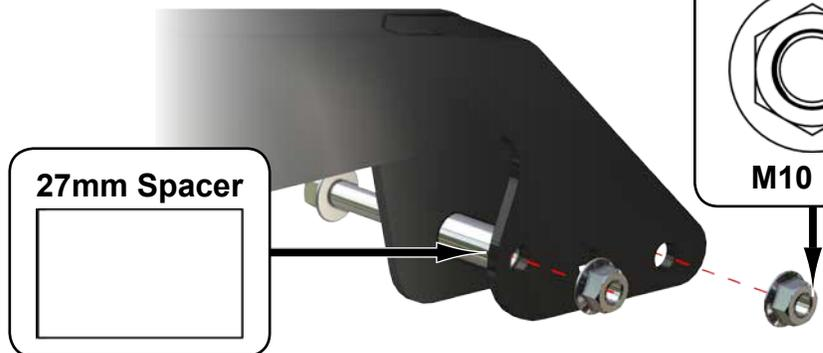
**Rear:** Keep all components removed from machine. Do not tighten hardware completely unless noted.
