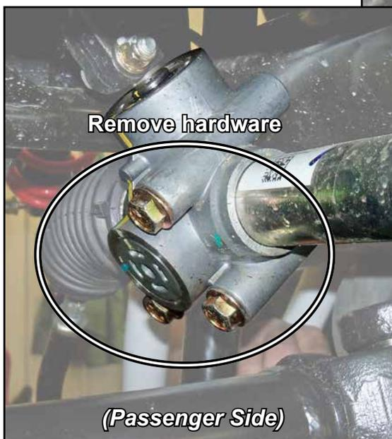
**Rack and Pinion Installation:** Do not tighten hardware completely unless noted.
