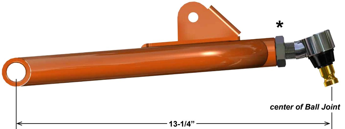
**\* Leave Jam Nuts loose. Tighten after final adjustments have been made.**
