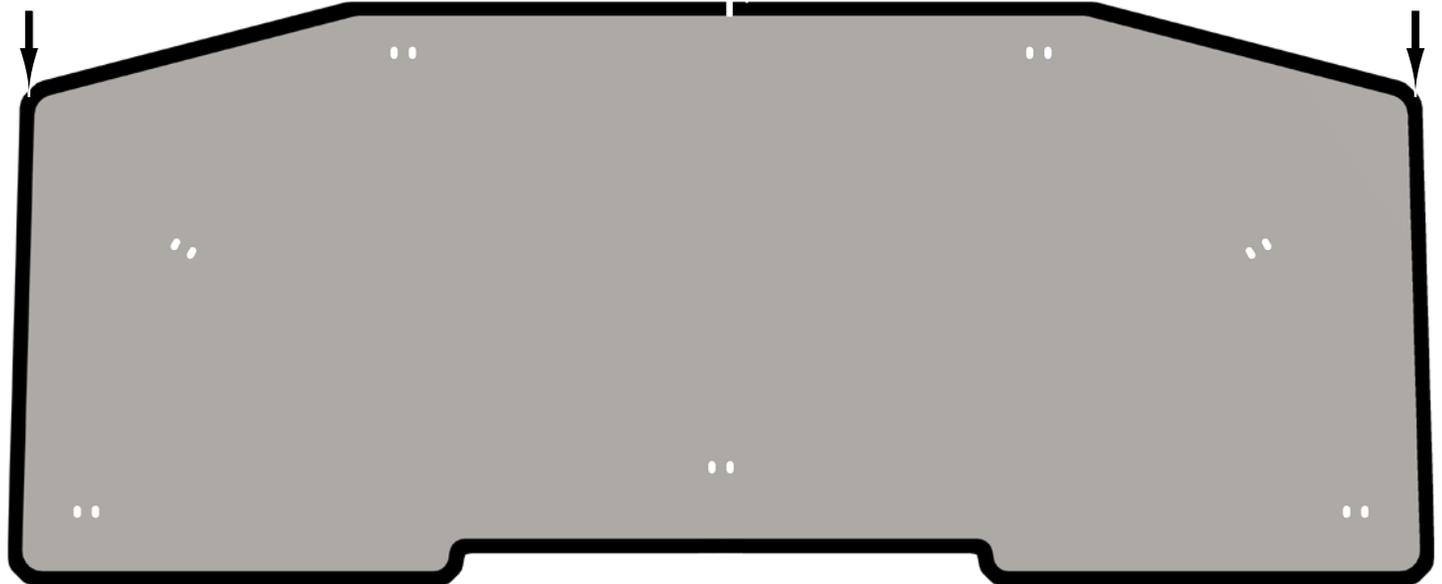
Soak Seal in hot water before cutting or installing to increase flexibility.
